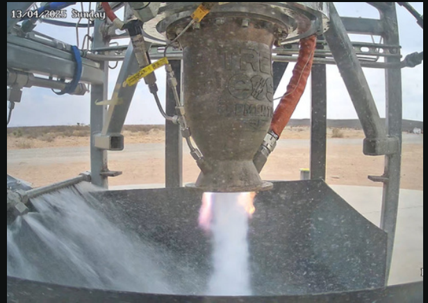
Largest student built rocket in the world to ever static fire
