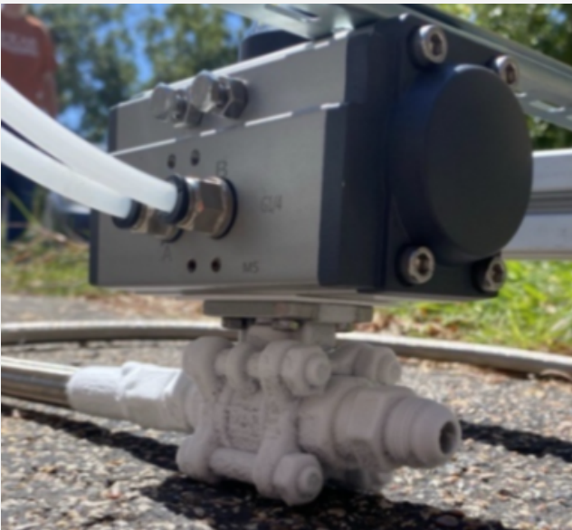
Image to the left: Valve immediately following a cryogenic beath
