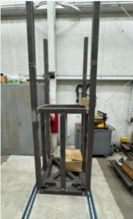
Image: Structural Test Stand for COPVs, cut and welded in-house
