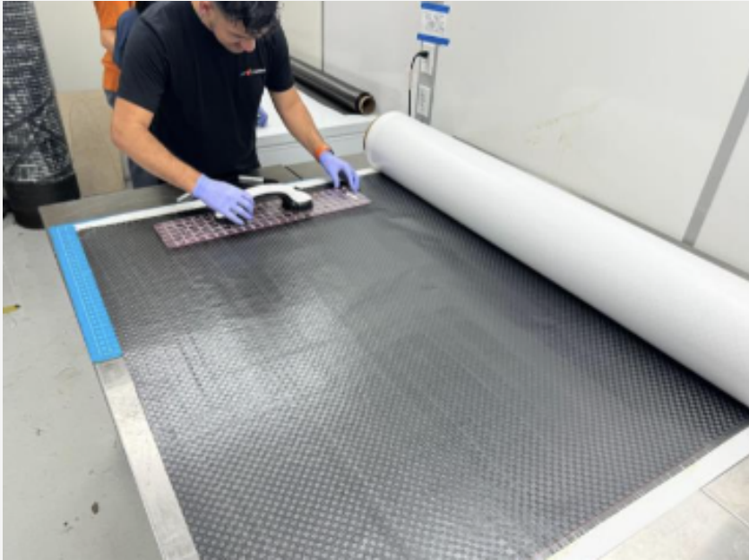
Image: Cutting sheets of pre-preg carbon fiber for Halcyon Mk1
