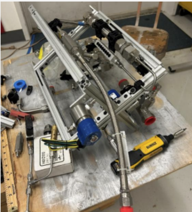
Image above: Halcyon engine bay fluids assembly in progress
