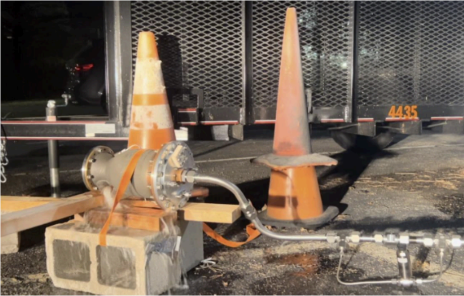
Image: Havoc SN2 (Mk2 engine, Mk1 backup) undergoing water flush testing of its regenerative cooling circuit post-manufacturing
