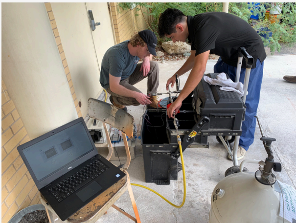
Image: Caelix Kidwell and Josue Renteria preparing for a purged dP testing with LN2.
