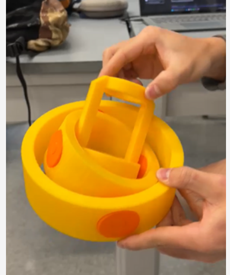
Image on the right: Zachary Handel demonstrates a concentric ring design for the pendulum's base.
