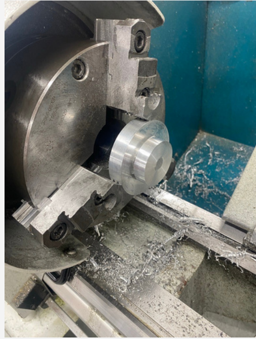
Image : Pump motor plate being turned on a lathe.
