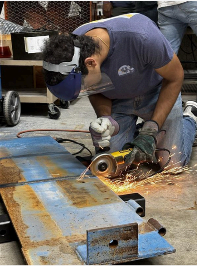
Image: Amogh Herle, Airframe Lead Engineer, cutting steel plate for use in compressive testing of composite skirts.
