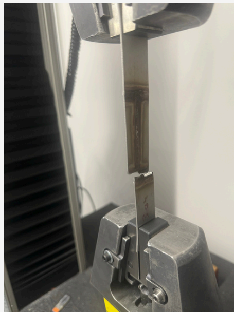
Image: “I” shaped weld failing at the bottom horizontal weld.
