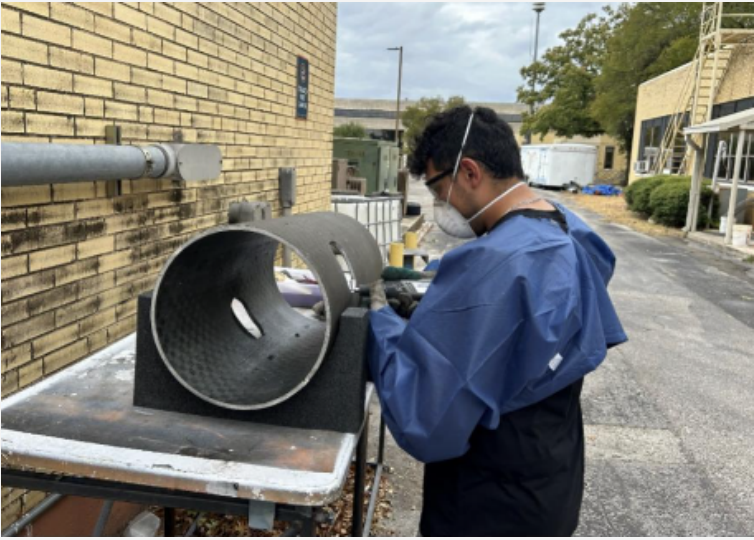
Image above: Structures manufacturing member Jose Juarez cleans up engine bay qualification skirt access port holes ahead of compression testing
