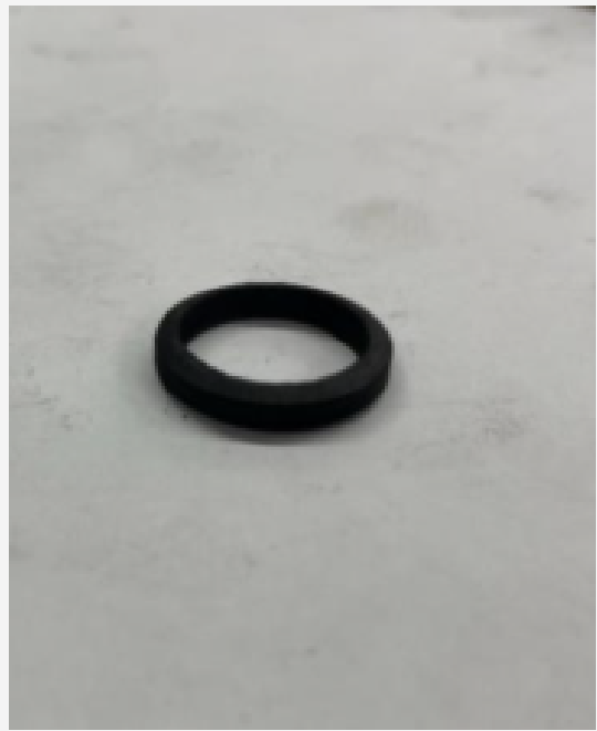
Image : Graphite ring used to seal the impeller shaft
