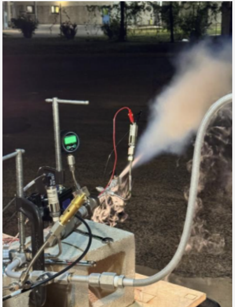
Image on the right: Liquid oxygen main valve cryogenic testing
