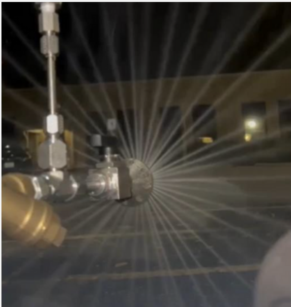
Images : Nemo pintle injector on the team's water flow cart
