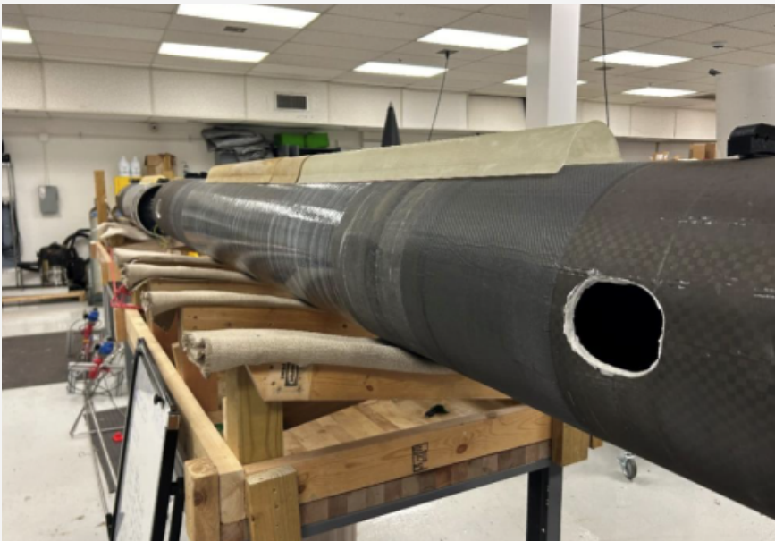
Image above : Halcyon Mk1 with fiberglass raceway covers positioned for fit checks
