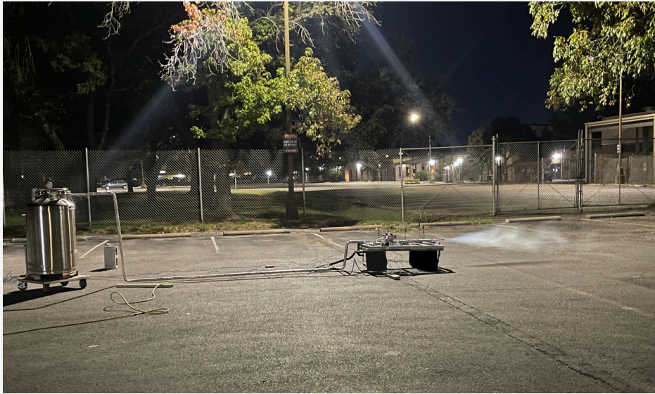
Image: Pump test cart fed by liquid nitrogen.
