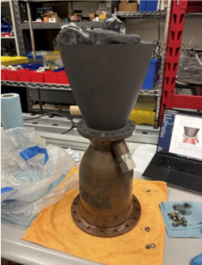
Image above: Havoc SN1 first full assembly with nozzle extension
