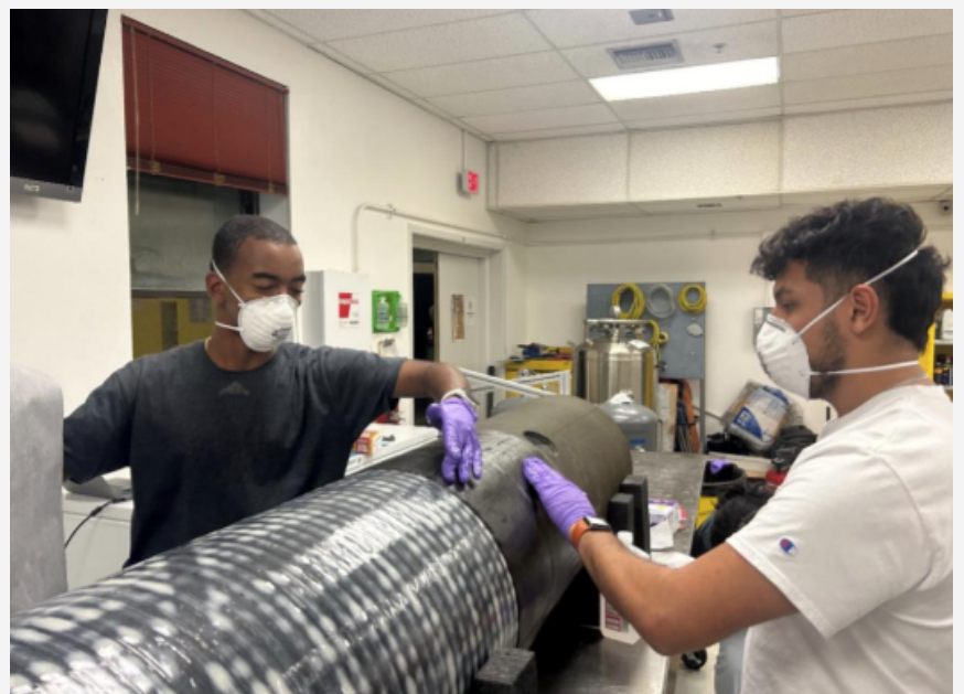
Image: Taj Lee (Head of Structures) and Jose Juarez (structures member) working on the engine bay skirt bond to the fuel tank
