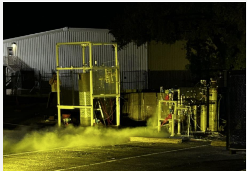
Image above: Halcyon GSE LOx fill system test
