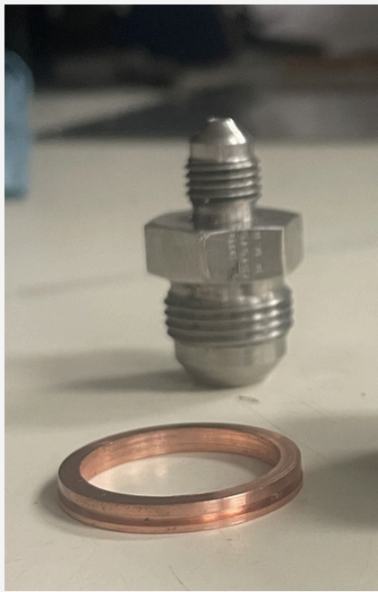
Image : Copper ring used on the LOX impeller
