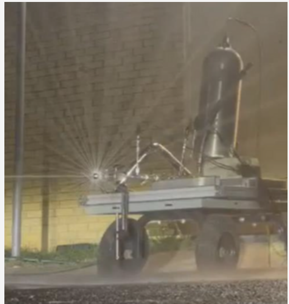
Images : Nemo pintle injector on the team's water flow cart
