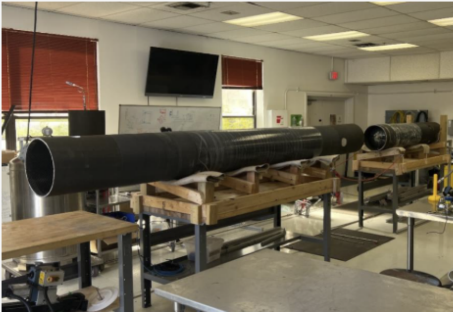
Image: Halcyon Mk1 with all carbon fiber composite work complete (sans some final cutouts in the forward LOx section)
