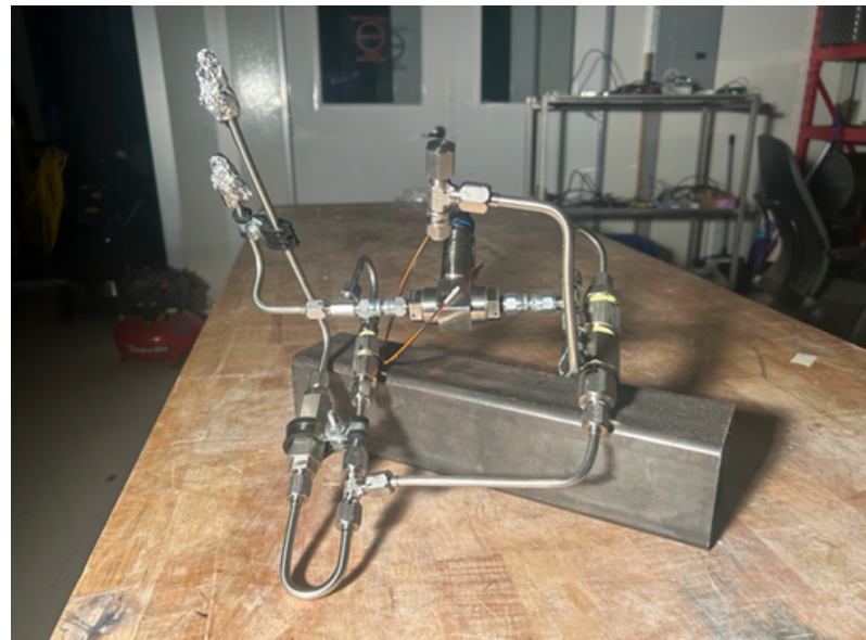
Image: Completed LOx tank forward assembly
