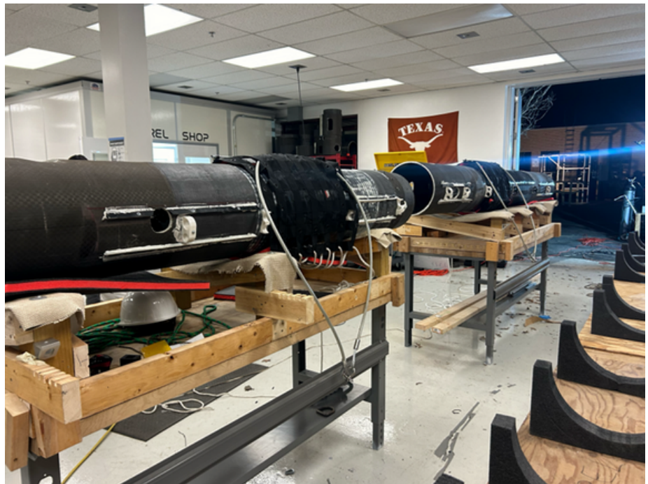
Image: Lift “corset” iterations prepped for the first dual-tank lift test attempt
