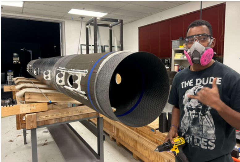
Image: Taj Lee installing the intertank composite coupler for the first time
