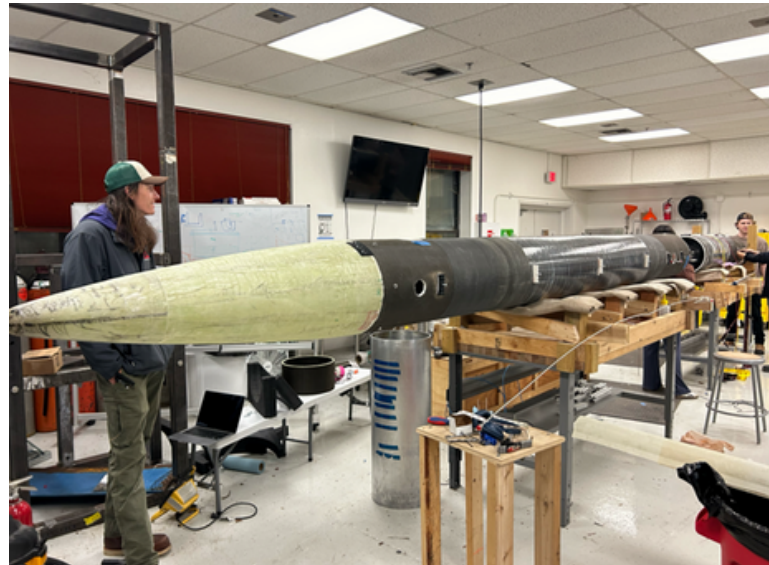
Image: First fiberglass nosecone integration
