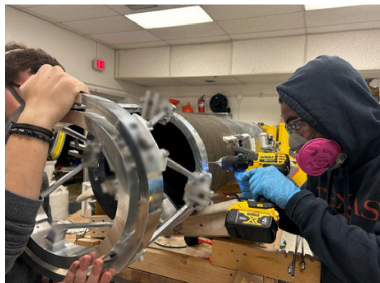
Image: Taj Lee and Daniel Brzostowski installing TVC assembly for the first time
